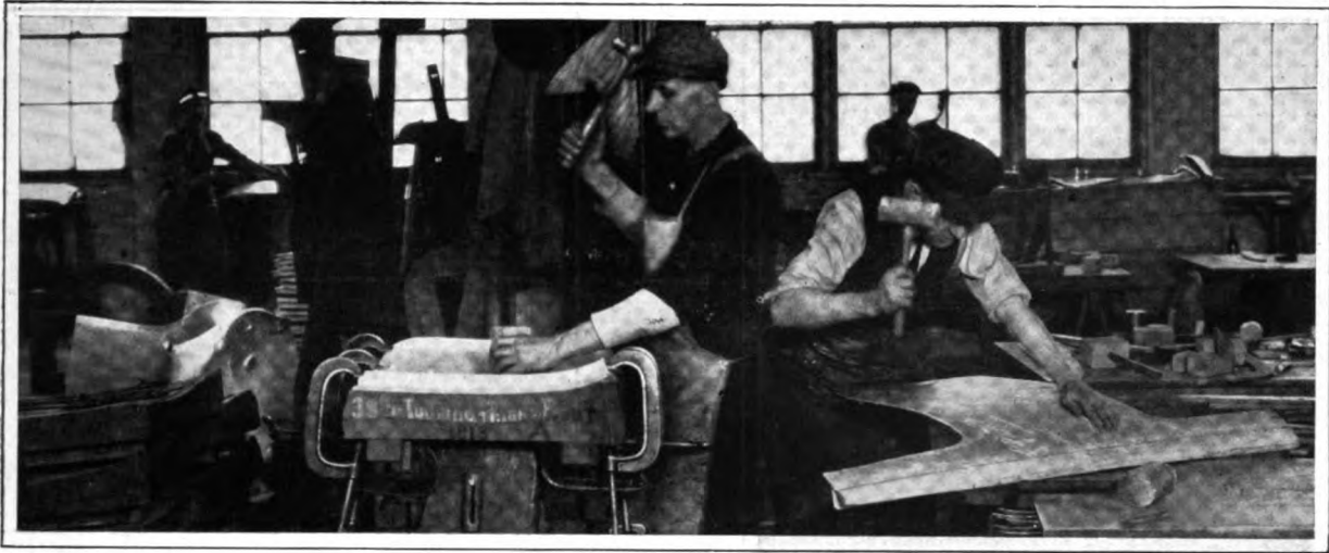
A photograph of the practice of hammering sections of aluminum castings for automobile bodies to fit wooden molds in the Pierce-Arrow plant
